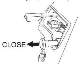
Figure 26. Choke Lever (Closed Position)
